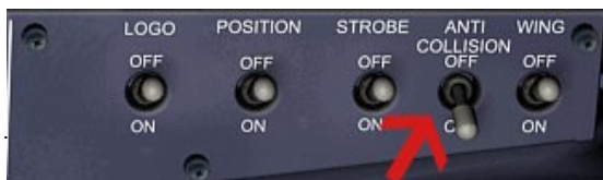
The Lightsystems are not that important, just be sure to turn on the BEACON LIGHT before engine startup
