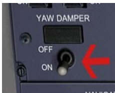
YAW DAMPER (as the name says, damps the yaw movements)... ON
