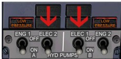
ENG&ELEC 1 & 2 Hydraulic Pumps (The hydraulics are one essential system of the plane)... ON
