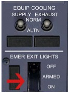
EMER EXIT LIGHTS (the emergency exit lights)..... ARMED
